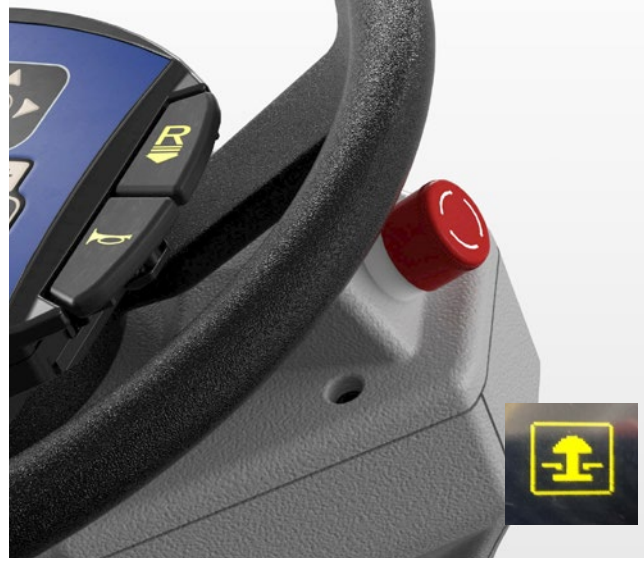
2. E-stop icon that appears on display when E-stop switch is engaged. Twist E-stop switch to enable machine function
