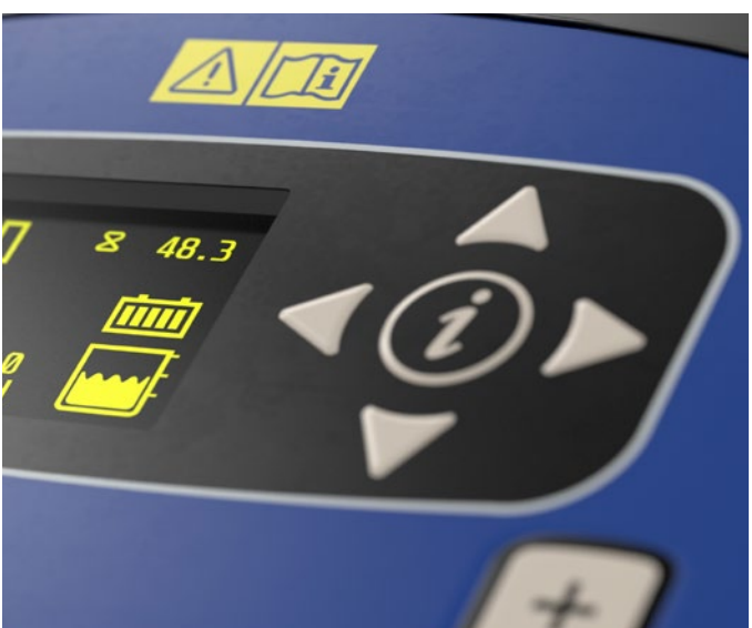
17. Press "I" scroll down to faults and press ">" button to view faults
