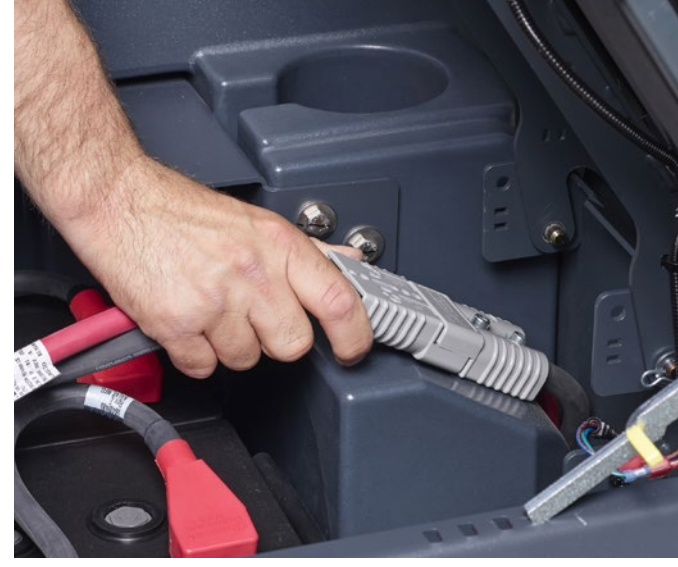
3. Check battery cables are well connected together
