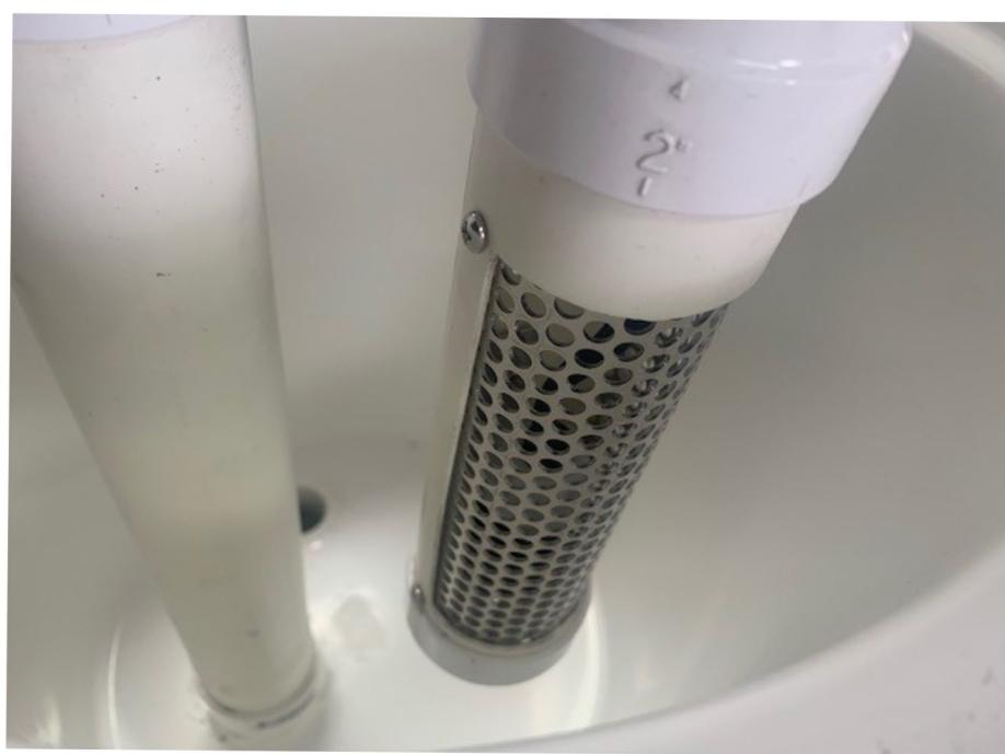
Pictured above is the water cut off system used in the Terminator plus. The Float switch cut off waste water from entering the vac motors.
