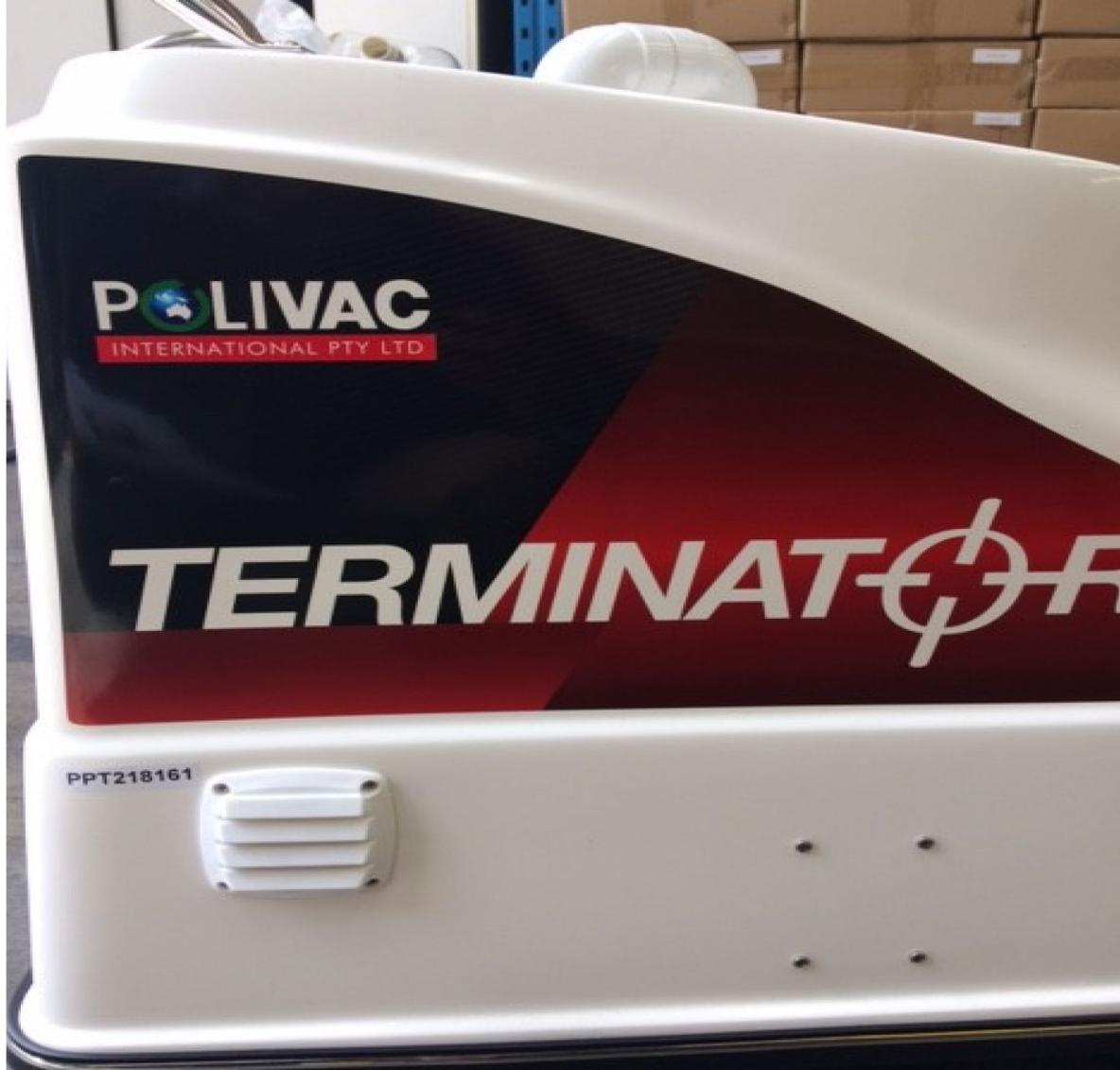
The above picture shows the exhaust point for the vacuum motors. If at any stage the operator experiences water coming from this point it indicates Foam is passing by the filter & this needs to be stopped. Water coming from this point Can only come thru the vac motors. To prevent foam build up, use an antifoaming Chemical agent. Do so by pouring a small amount of antifoam solution directly into Waste tank prior to steam cleaning.
