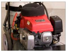
A 12 volt push-button start, fires the 13hp (9.69 kw), 4 stroke overhead valve Honda engine into action while the brushes are on the floor.
