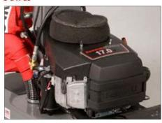
The 18 horsepower Kawasaki motor ensures consistent power delivery to the pads for even and patch-free finish.
