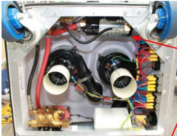
Mount the pump to the internal wall using nuts provided
